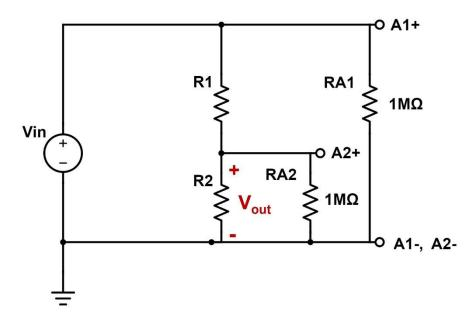
Under which conditions do we need to be concerned that the input impedance of channel 2 (RA2) will noticeably affect the voltage measurement across R2?
