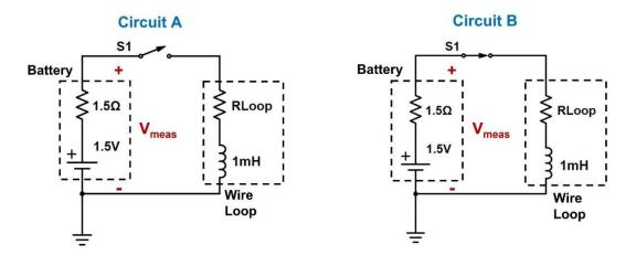
If the voltage across the battery is measured while the motor is operating, the plot below is observed on the oscilloscope: when the circuit is open (A), 1.5 V is measured across the battery and when the circuit is closed (B), 0.75 V is measured.
