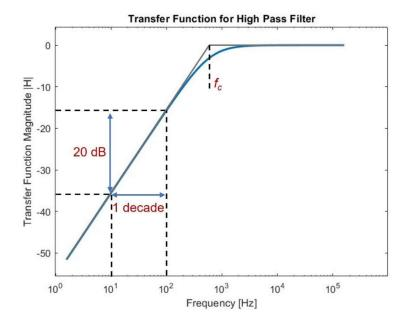
**a.)** (4 pts) To filter out the 60 Hz noise, we want to design a high pass filter whose attenuation at f = 60 Hz is 40 dB (i.e.,  $|H(j\omega)| = -40$  dB at 60 Hz). Assuming that the corner frequency  $f_c$  is located where the linear approximation of the filter at low frequencies crosses 0 dB (as in the plot above), what corner frequency (in Hz) should the high pass filter we are designing have?
