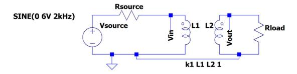
Assume L1 and L2 form an ideal transformer with full coupling. The transformer has these specifications: a=3, L1=5mH
