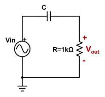
Using the value determined for the corner frequency in Q2.1, calculate the capacitance C required for the filter.
