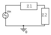
This circuit shown above has 2 complex impedances, Z1 and Z2, connected as shown.
