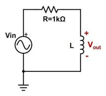
What value of L is required to implement a high-pass filter with the same corner frequency as calculated in Q2.1?
