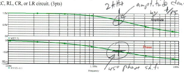
1) Is this a low pass or high pass filter? Circle one: Low Pass High Pass
