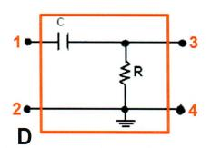
a) Shown above are the four basic, two-element, passive filter configurations made with RL and RC combinations. Determine the general complex transfer function for each circuit in terms of R, L, C and frequency ω, by modeling each as a voltage divider. (4 pts)
