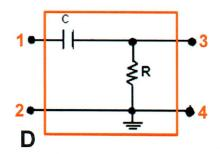
a) Shown above are the four basic, two-element, passive filter configurations made with RL and RC combinations. Determine the general complex transfer function for each circuit in terms of R, L, C and frequency  $\omega$ , by modeling each as a voltage divider. (4 pts)
