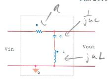
1. Write the transfer function for Vout/Vin as a ratio of polynomials. (2pts)
