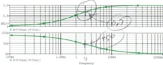
1) Is this a low pass or high pass filter? Circle one: Low Pass
