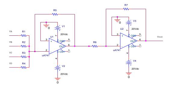
a) Select values for R1, R2, R3, and R4 so that the output voltage will be the decimal equivalent of ABCD. For example, if ABCD=1010, or equivalently VA=VC=5 V, VB=VD=0 V, then Vout = 10 V. The circuit should work for <u>all</u> possible ABCD combinations. (12 points)
