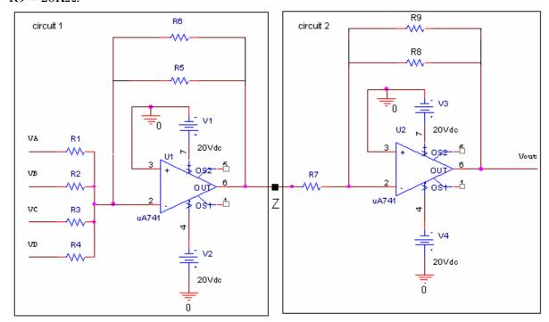
a) What kind of circuit is circuit 1? Give an equation for the output of circuit 1 at point Z in terms of VA, VB, VC, and VD. Substitute numerical values for the known reistances, but leave in terms of the unknown resistances: R1, R2, R3 and R4. (4 points)
