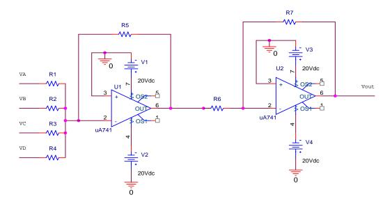
a) Select values for R1, R2, R3, and R4 so that the output voltage will be the decimal equivalent of DCBA. For example, if DCBA=1010, or equivalently VD=VB=5 V, VA=VC=0 V, then Vout = 10 V. The circuit should work for <u>all</u> possible DCBA combinations. (12 points)
