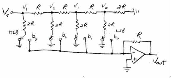
The digital input to the DAC is a 4-bit binary number represented by bits b0, b1, b2 and b3, where b0 is the least significant bit (LSB) and b3 is the most significant bit (MSB). Each bit in the circuit controls a switch between ground and the *inverting* input op amp. When a bit is 1, the corresponding switch is connected to the op-amp; when a bit is zero, the corresponding switch is connected to ground.
