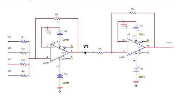
a) Select values for R1, R2, R3, and R4 so that the output voltage will be the decimal equivalent of DCBA. For example, if DCBA=1010, or equivalently VD=VB=5 V, VA=VC=0 V, then Vout = 10 V. The circuit should work for <u>all</u> possible DCBA combinations. (12 points)
