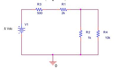
In the circuit above, V1=5 volts. R1=  $2000\Omega$ , R2=  $1000\Omega$ , R3=  $500\Omega$ , R4=  $10,000\Omega$
