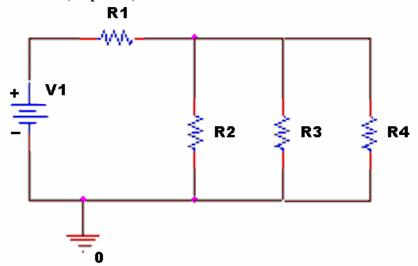
In the circuit above, V1=5 volts. R1=  $50\Omega$ , R2=  $1000\Omega$ , R3=  $2000\Omega$ , R4=  $3000\Omega$
