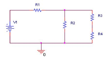
Given: V1=5 volts. R1=  $2000\Omega$ , R2=  $1000\Omega$ , R3=  $500\Omega$ , R4=  $400\Omega$
