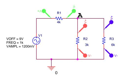
a) Given the circuit above, calculate the DC offset voltage at point A. (5 points)
