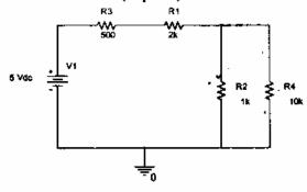
In the circuit above, V1=5 volts. R1=  $2000\Omega$ , K2=  $1000\Omega$ , R3=  $500\Omega$ , R4=  $10,000\Omega$
