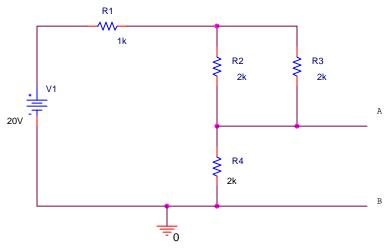
In the circuit above, determine the voltage between the two points marked A and B.
