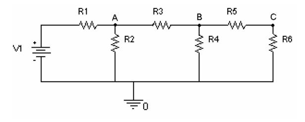
a) Find the combined resistance of the circuit with respect to V1. (6 points)
