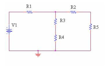
Given: V1=5 volts. R1=  $50\Omega$ , R2=  $3000\Omega$ , R3=  $1000\Omega$ , R4=  $550\Omega$ , R5= $440\Omega$
