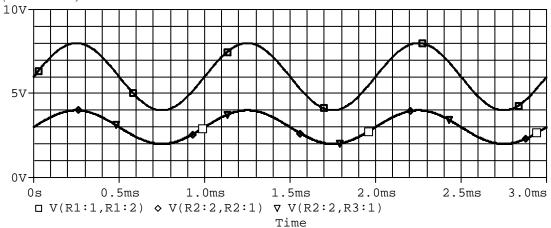
The plot below is correct. The DC voltage is 6V for R1 (square), and 3V for R2 and R3 (triangle and diamond). The amplitude across R1 is about 0.8V and over R2 and R3 is half that. The voltage across R2 and R3 must be the same because they are in parallel.
