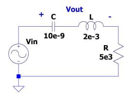
b. [4 pts] Sketch a plot of |H(jω)| on a log-linear scale. You must show your work in evaluating H(jω) in the limit of very low frequencies and very high frequencies. Label all relevant filter frequency parameters (corner frequency/frequencies, center frequency, etc.) on the plot. Note: You do not need to give numerical frequencies for any corner frequencies, but you must give a numerical frequency for a center frequency (if applicable to your filter).
