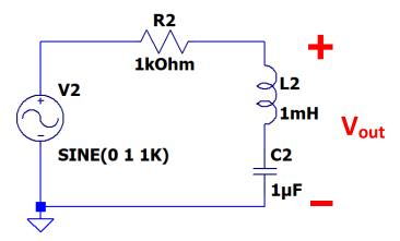
a) [4 pts] Find the transfer function H(s) of the circuit above for the Vout indicated in the circuit diagram. Rearrange your expression for H(s) so that the denominator takes the form:  $s^2 + \alpha s + \beta$ , where  $\alpha$  and  $\beta$  are constants. Then, also write your transfer function in terms of j $\omega$  to give H(j $\omega$ ).
