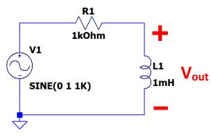
a) [2 pts] Redraw the circuit above in terms of the impedances  $Z_{R1}$  and  $Z_{L1}$ . Also write the expressions for the impedance of each element (in terms of R1, L1 and s) next to the appropriate element in the diagram.
