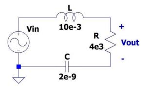
b. [4 pts] Sketch a plot of |H(jω)| on a log-linear scale. You must show your work in evaluating H(jω) in the limit of very low frequencies and very high frequencies. Label all relevant filter frequency parameters (corner frequency/frequencies, center frequency, etc.) on the plot. Note: You do not need to give numerical frequencies for any corner frequencies, but you must give a numerical frequency for a center frequency (if applicable to your filter).
