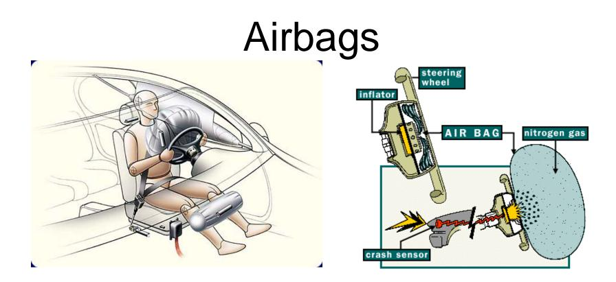
Several types of accelerometers are used & at least 2 must sense excessive acceleration to trigger the airbag.
