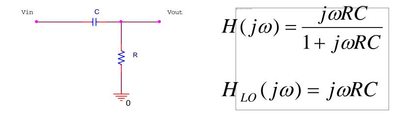
$$V_{out} = V_R = RC \frac{dV_C}{dt} \approx RC \frac{dV_{in}}{dt}$$
