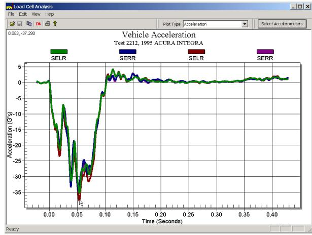
Ballpark Calc: 56.6mph = 25.3m/s Stopping in 0.1 s Acceleration is about  $-253 \text{ m/s}^2 = -25.8 \text{ g}$
