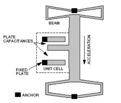
Simplified View of Sensor Under Acceleration
