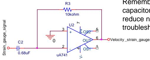
Remember that a feedback capacitor is probably necessary to reduce noise on the signal. See troubleshooting guide.
