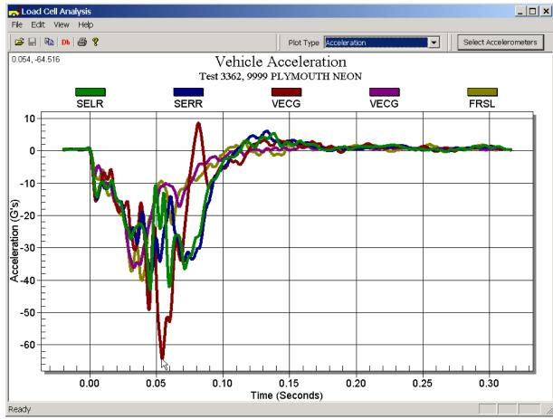
Ballpark Calc: 112.1mph = 50.1 m/s Stopping in 0.1 s Acceleration is about  $-501 \text{ m/s}^2 = -51.1 \text{ g}$
