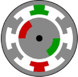
• A brushless dc motor has a rotor with permanent magnets and a stator with windings. It is essentially a dc motor turned inside out. The control electronics replace the function of the commutator and energize the proper winding.
