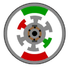
• Just as the rotor reaches alignment, the brushes move across the commutator contacts and energize the next winding. In the animation the commutator contacts are brown and the brushes are dark grey. A yellow spark shows when the brushes switch to the next winding.
