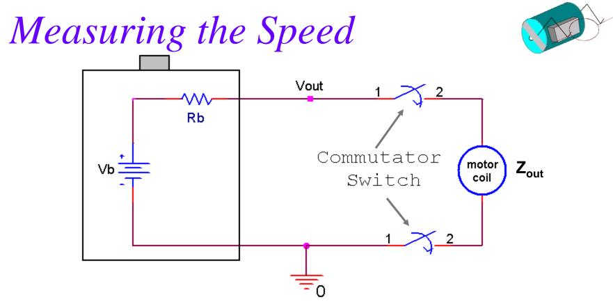
• As the coil rotates, it connects to the power supply about half the time. When this occurs, the voltage measured at the battery or power supply will drop (voltage divider action). Thus, a series of pulses will be observed, which can be used to determine the frequency of revolution.
