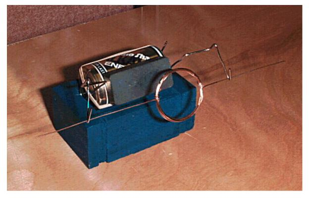
• A simple DC motor with brushes made with a battery, two paperclips, a rubber band and about 1 meter of enameled wire.
