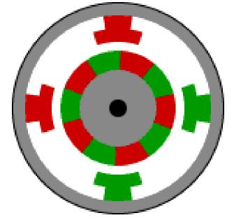
This animation shows the stepping pattern for a half-step stepper motor. The commutation sequence for a half-step stepper motor has eight steps instead of four. The main difference is that the second phase is turned on before the first phase is turned off. Thus, sometimes both phases are energized at the same time. During the half-steps the rotor is held in between the two full-step positions. A half-step motor has twice the resolution of a full step motor. It is very popular for this reason.
