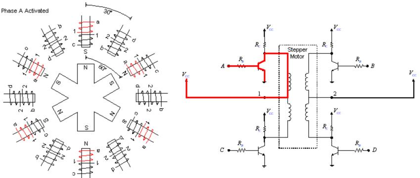
Note how the phases are driven so that the rotor takes half steps
