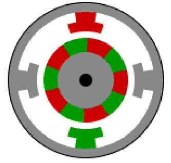
This animation demonstrates the principle for a stepper motor using full step commutation. The rotor of a permanent magnet stepper motor consists of permanent magnets and the stator has two pairs of windings. Just as the rotor aligns with one of the stator poles, the second phase is energized. The two phases alternate on and off and also reverse polarity. There are four steps. One phase lags the other phase by one step. This is equivalent to one forth of an electrical cycle or 90°.
