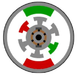
• The stator is the stationary outside part of a motor. The rotor is the inner part which rotates. In the motor animations, red represents a magnet or winding with a north polarization, while green represents a magnet or winding with a south polarization. Opposite, red and green, polarities attract.
