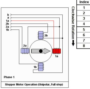
Full step sequence showing how binary numbers can control the motor
