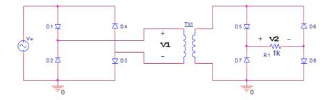
3.c) (3 pts) If the frequency of Vin is 1 kHz and it has an amplitude of 20 V, what is the dominant frequency of the output of the first rectifier, V1? Also, what is the dominant frequency of the signal being applied to the load resistor, V2?
