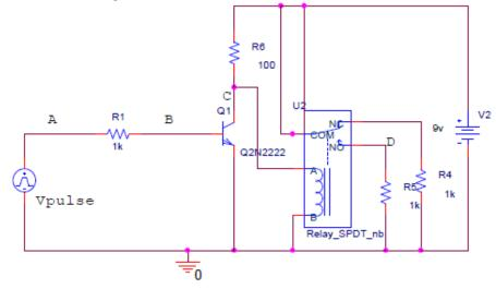
In the circuit above, the voltage source Vpulse puts out a sequence of pulses and the voltages at the source and three other points are monitored (marked A, B, C, and D). The relay model used by PSpice lists *the resistance of the coil to be 100 ohms (This is important!*):
