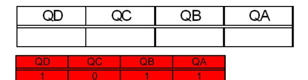
3. A 4-bit counter is cleared and then receives a string of clock pulses. What are QA, QB, QC and QD after 21 clock pulses? Clearly indicate the state of each signal. (*2pts*)
