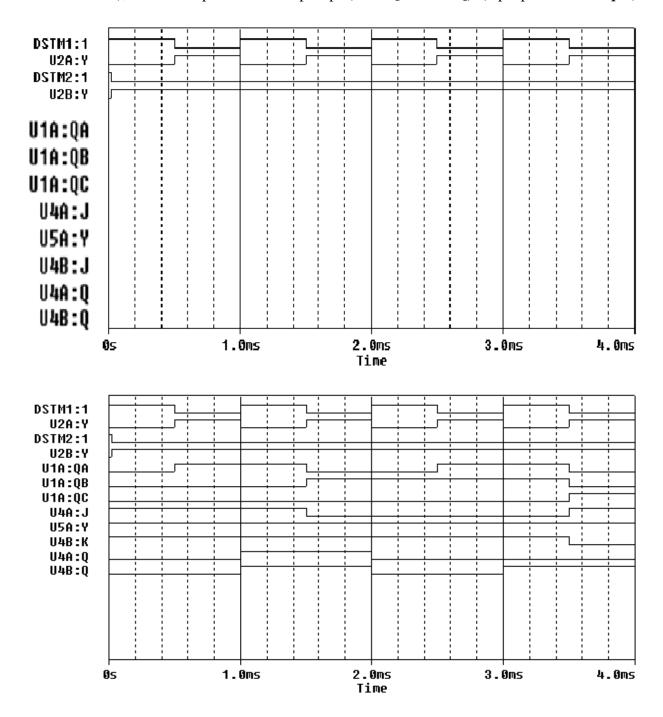
2. A 4-bit counter is cleared and then receives a string of clock pulses. What are QA, QB, QC and QD after 11 clock pulses? Clearly indicate the state of each signal. (*2 pts*)
