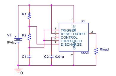
2. (4pt) Using a ratio from above and  $C1 = 1\mu F$ , calculate the values for R1 and R2 needed to yield a frequency of 440Hz.
