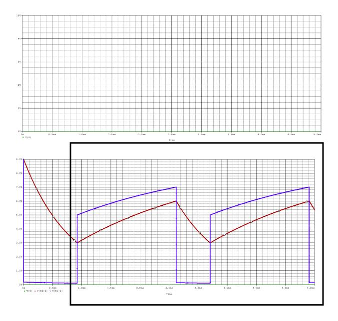
PSpice was used to generate the plot. Only the part in the box is required for this answer. The first part of the signal is an artifact of the way PSpice initializes voltages.
