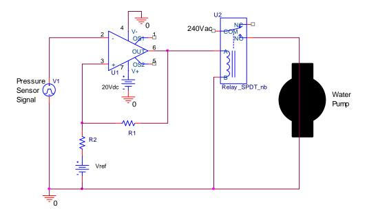
2. (3pt) Given a tank pressure sensor transducer circuit that outputs 0.5V/psi (V1 in the above circuit), what would be appropriate voltage thresholds for the high power ideal op-amp circuit to match the pump's two switching points?
