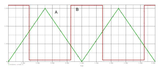
A: Triangular wave rising from zero to 3V and back in 1ms, which is what the vpulse is set up to do. B: The triangular wave triggers the Schmitt trigger at around 1.7V and about 0.8V which is what it is designed to do. The output voltage goes high when triggered on (above 3V) and low (near zero) when off. The hysteresis of the Schmitt trigger is clear from these different levels.
