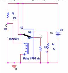
VD = 9V $VC = V2*R_{relay}/(R_{relay} + R6) = 9(100)/(100+100) = 4.5V$
