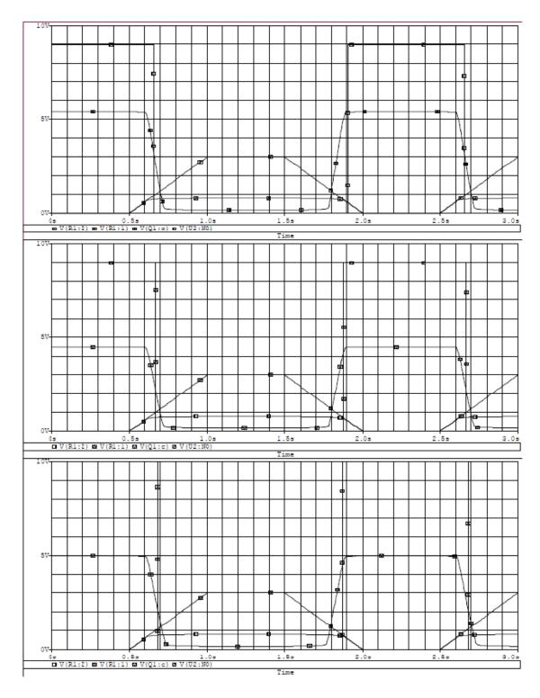
Answer: Vpulse is off(0 volts)  $\ll VA = 0V$  (pulse low) and VB = 0V (pulse low)  $\ll$  diode is off  $\ll$ current flows through relay  $\ll$  relay switch at NO
