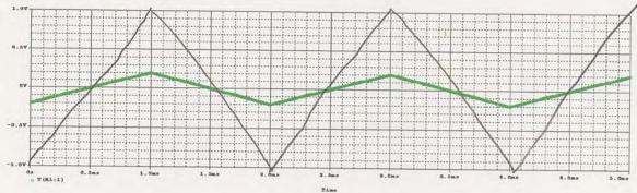
d. {4 pts} The input voltage is shown below. Solve for and sketch the output voltage for circuit C with R=2kΩ and C=0.047μF. (Extra Credit)
