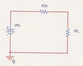
The Thevenin equivalent circuit consists of a voltage source in series with a resistor, which provides a very simple replacement for much more complex circuits. If we have this simple source, analyzing changing loads becomes quite easy.
