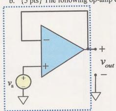
Determine the Thevenin equivalent voltage  $V_{TH}$  and the The venin equivalent resistance  $R_{TH}$  for this circuit including the source  $v_s$  (that is, everything inside the dashed box).
