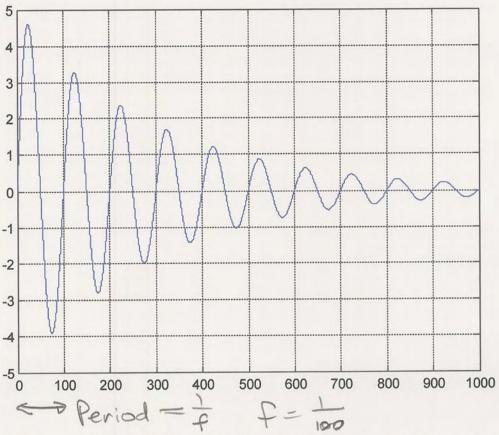
where the horizontal scale is time (100 sec per division) and the vertical scale is velocity (1 m/s per division).
