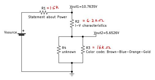
i. The power absorbed by resistor R1 is 4.3 mW when 1.693 mA flows through it. What is the value of R1? (1pt) *Use the closest standard resistor value; refer to information on "Standard Resistor Values" at the beginning of the quiz.*
