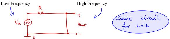
**d.** Corner frequency of a filter,  $f_c$ , is defined as the frequency at which the magnitude of the transfer function,  $|H(j\omega)|$ , is 0.707, or  $\frac{1}{\sqrt{2}}$ . Alternatively, this can be expressed as the frequency at which the power at the output is half of the power at the input. **Derive the corner frequency or frequencies** for this circuit when  $R=10 \Omega$ , L=2H, and C=0.5F? (5 pts)
