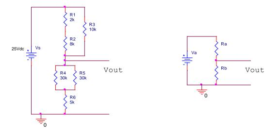
R1, R2, and R3 all compose Ra. First find the series total of R1 and R2, then the parallel value including R3:
