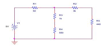
R2 and R5 are in series, replace with "R25," and R3 and R4 are in series, replace with "R34":
