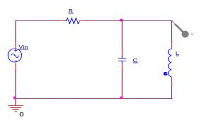
3.d) (4 pnts) Find the transfer function of the circuit, simplified such that there are no fractions in the numerator or denominator of the transfer function.
