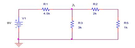
1.a) (6 pnts) What is the voltage at point A in the circuit above?
