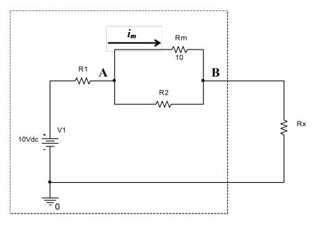
**Case 1**: Given that when  $Rx = 0 \Omega$ , the current through resistor Rm is 2 mA, i.e.  $i_m = 2$  mA. **Case 2**: Given that when  $Rx = 2000 \Omega$ , the current through resistor Rm is 1 mA, i.e.  $i_m = 1$  mA.
