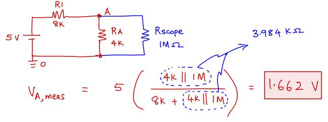
**g.** (4 pts) You are now asked to change R1 from  $8k\Omega$  to a new value such that the current through resistor R1 is close to 30 ptA. Voltage source V1 is set to 5V. What is your new choice of R1?
