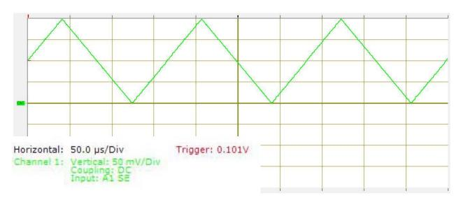
3 cycles in 10x50us so the frequency is 3/0.5ms=6kHz, the period is 0.5ms/3=1.67ms p-p amplitude is 4x50mV or 200mV or 0.2V, offset is 2x50mV or 100mV or 0.1V
