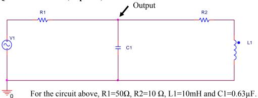
1) Which of the 3 graphs below would best represent the output seen across capacitor C1; where Vin = 120V  $cos(2\pi ft)$ , with **f** = **60Hz**? (8 pts)
