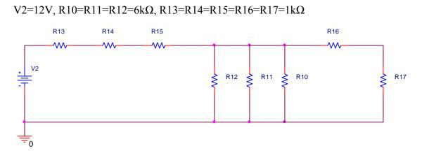
1) Find the total resistance of the circuit, seen from the voltage source. (6 pts)
