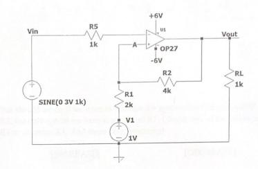
a. [2 pts] What is the functional name of this circuit, which utilizes the basic comparator operation of an op-amp?
