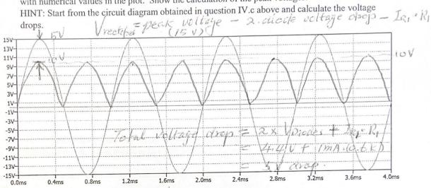
e. [4 pts] As shown in the circuit diagram below, we have added two **Green LEDs** between Vout nodes A and B to limit the voltage output. Sketch and label the voltage output between A and B in the plot below. Clearly label the peak voltages with numerical values and show your reasoning.
