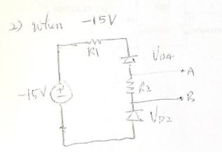
$I_{R1} = -15V + 2.(2.2V)$   $R_1 + R_2$  $= \frac{-10.6V}{10.6K02}$ =  $\left[-1 m A\right]$
