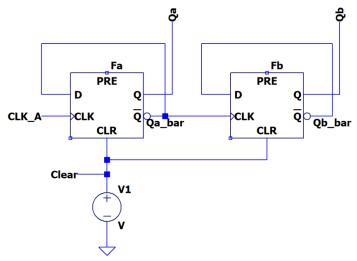
Complete the timing diagram below by sketching the outputs  $Q_a$ ,  $\overline{Q_a}$  (Qa\_bar),  $Q_b$  and  $\overline{Q_b}$  (Qb\_bar). Hint: begin with  $Q_a$  and  $\overline{Q_a}$  (Qa\_bar).
