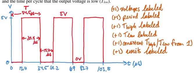
3. [2 pts] Calculate the duty cycle of the output of the 555 timer.
