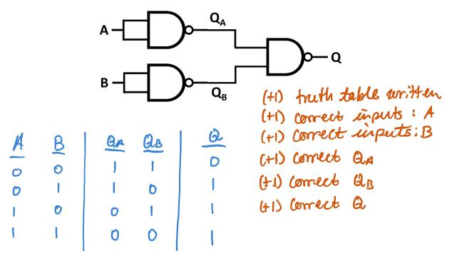
2. [2 pts] To which fundamental 2-input logic gate is the circuit in part 1 equivalent? Explain your reasoning in one sentence.
