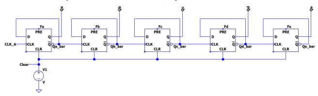
This circuit is a 5-bit counter, which could represent a largest number (in binary) of **11111**. The decimal representation of 11111 is  $1*2^0 + 1*2^1 + 1*2^2 + 1*2^3 + 1*2^4 = 1 + 2 + 4 + 8 + 16 = 31$
