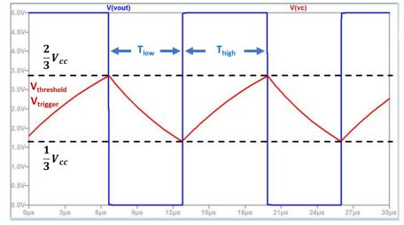
Why is  $T_{high}$  determined by  $(R_1+R_2)C_1$ , but  $T_{low}$  is determined by  $R_2C_1$ ?
