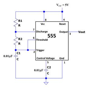
1. (4 pts) You are tasked with using the 555 timer to generate a train of voltage pulses with a frequency of f = 100 kHz and a duty cycle of 75%. Calculate the total period of one cycle of pulses (*T*), the amount of time per cycle that the voltage output is high (*T*<sub>high</sub>) and the amount of time per cycle that the voltage output is low (*T*<sub>low</sub>).
