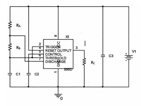
**a.** (4 pts) The 555 astable multivibrator circuit shown above is to have a duty cycle of 75%. What ratio of resistors R1/R2 will produce this duty cycle?
