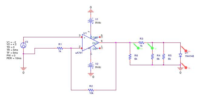
Note the three  $6k\Omega$  Ohm resistors placed from the measurement points to ground. These  $6k\Omega$  resistors represent the input impedance of the Mobile Studio board.
