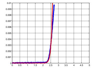
*K.A. Connor* Rensselaer Polytechnic Institute Note that this approach does indeed get rid of the finite slope data in the part of the curve near the horizontal axis. The differences between the measured data and the ideal equation are due to some additional losses that occur in LEDs that we do not see in conventional diodes like the 1N4148.
