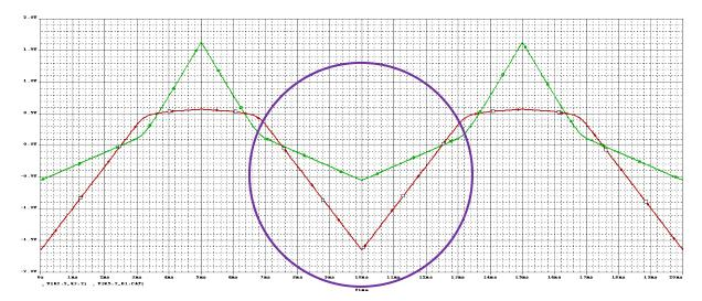
The purple circle shows the problem area. When the diode is reverse biased, it will carry no current. However, the 6k resistors can carry current, which will distort the data. If we replace the 6k resistors with 10 Meg resistors (corresponding to the input impedance of the lower voltage ranges, such as 500mV/div), we get an undistorted picture of what a diode does.
