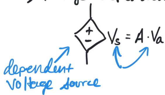
Voltage supplied by source depends on a voltage somewhere else in the circuit
