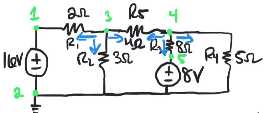
$$\text{Node 3: } \frac{V_3 - 16}{R_1} + \frac{V_3}{R_2} + \frac{V_3 - V_4}{R_5} = 0$$
