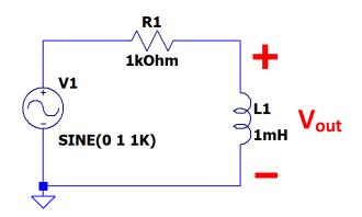
a) [2 pts] Redraw the circuit above in terms of the impedances Z<sub>R1</sub> and Z<sub>L1</sub>. Also write the expressions for the impedance of each element (in terms of R1, L1 and s) next to the appropriate element in the diagram.
