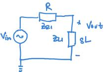
b) [4 pts] Find the transfer function H(s) of the circuit above for the Vout indicated in the circuit diagram. Rearrange your expression for H(s) so that the denominator takes the form:  $s + \alpha$ , where  $\alpha$  is a constant. Then, also write your transfer function in terms of j $\omega$  to give H(j $\omega$ ).
