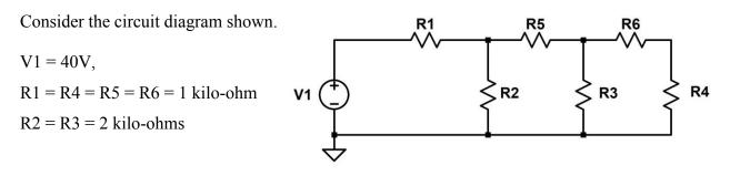
Part a) (3 points) Find the total resistance of the circuit, seen from the voltage source.
