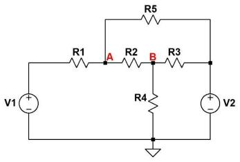
**Part b)** (10 points) Use nodal analysis to find the matrix equation,  $A\mathbf{x} = \mathbf{b}$ . All your terms should be symbolic (no numbers needed). Your final answer should be expressed as a matrix equation as shown below.  $V_A$  and  $V_B$  are nodal voltages at nodes A and B respectively.
