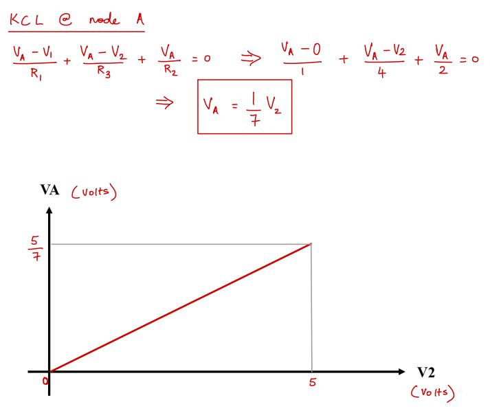
Based on the above results for the two source circuit, determine the voltage at node A when V1 = 4 V and V2 = 2 V.
