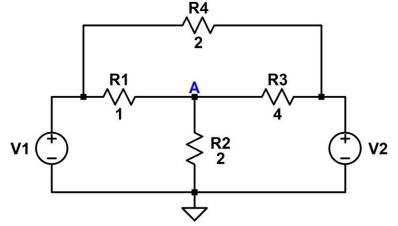
The voltage at V2 was set to zero and the voltage V1 was swept from 0 to 5V. Sketch the voltage at node A to plot VA vs. V1 (with V2 = 0) in the graph below. Label axes clearly.
