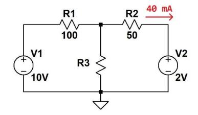
**Part a)** (10 points) Determine the value of resistance R3 using nodal analysis such that the current through R2 is 40 mA as shown. Show handwritten work.
