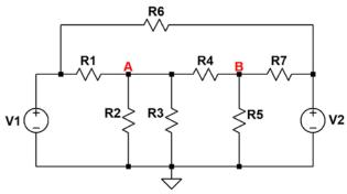
**Part b)** (10 points) Use nodal analysis to find the matrix equation, Ax = b. All your terms should be symbolic (no numbers needed). Your final answer should be expressed as a matrix equation as shown below.  $V_A$  and  $V_B$  are nodal voltages at nodes A and B respectively.
