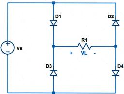
c) For the above circuit, assuming the diodes are ideal with VTurn-on = 1V, sketch the voltage across the resistor. (5 pts)
