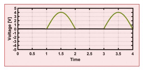
b) For the same circuit on the previous page (part a circuit), assuming the diode is ideal with VTurn-on = 1V, sketch the voltage across the resistor. (3 pts)
