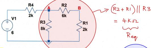
a) Use any method to find the voltages at nodes A and B. (6 pts)
