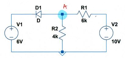
The diode in the above circuit is ideal, with  $V_{Turn-on} = 1V$ . (Same circuit as the previous page.)
