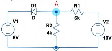
The diode in the above circuit is ideal, with  $V_{Turn-on} = 1V$ .
