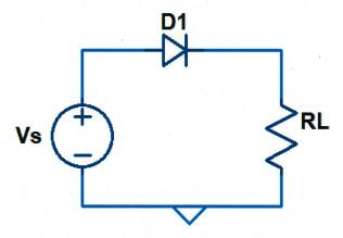
a) For the above circuit, assuming the diode is ideal with VTurn-on = 0V, sketch the voltage across the resistor. (3 pts)
