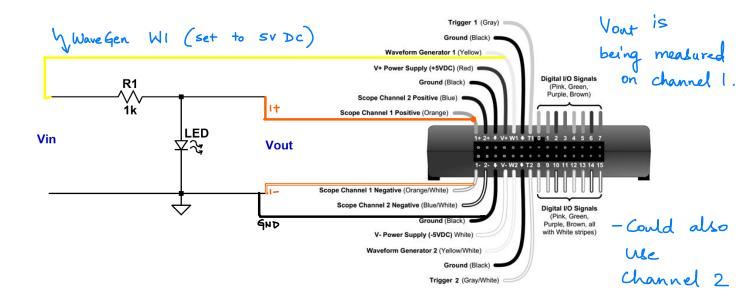
b) If your measurement for Vout is 2.0V (when Vin is 5V), find the current that flows through the resistor R1. (2 pts)
