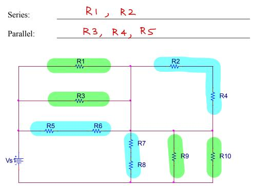
b) For the above circuit, indicate which **pairs** of resistors are in series and which resistors are in parallel. Each line is for a specific pair. There may be more lines than needed. (8 pts)
