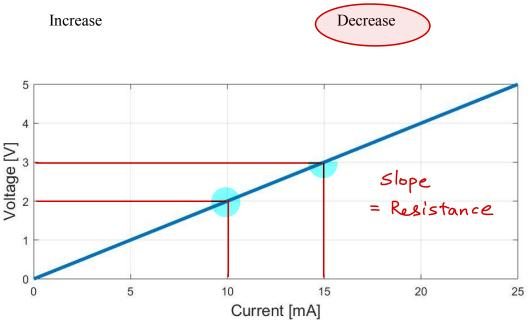
The above linear plot relates voltage and current in a resistor (similar to the circuit at the top of the page).
