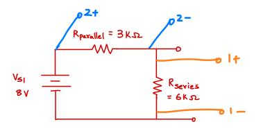
e) Use your simplified circuit to determine the voltages across the equivalent resistors, Rseries and Rparallel, as indicated by the Channel 1 and 2 connections in the original circuit. (4 pts)
