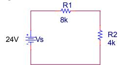
a) For the above circuit, determine the voltages across R1 and R2. (4 pts)
