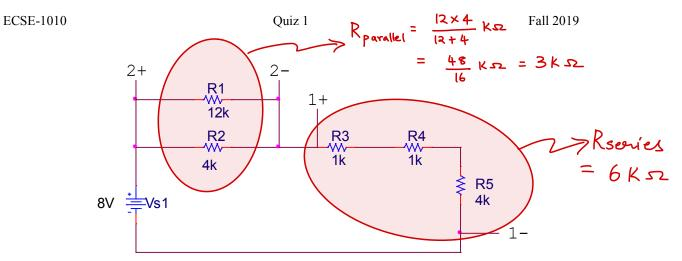
d) Apply series and parallel relationships to obtain a simplified two resistor (Rseries and Rparallel) circuit. Sketch the new circuit. (4 pts)
