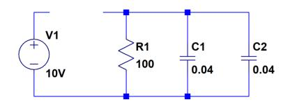
In the above circuit, the voltage source is connected to the circuit and then disconnected at t = 0s (time equals zero). Additionally, at t = 5s, capacitor C2 is disconnected from the circuit, discharged by shorting the leads and then immediately reconnected to the circuit (all happening very quickly). To the best of your artistic ability, sketch the voltage across capacitor C1 as a function of time.
