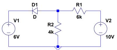
The diode in the above circuit is ideal, with  $V_{Turn-on} = 1V$ .
