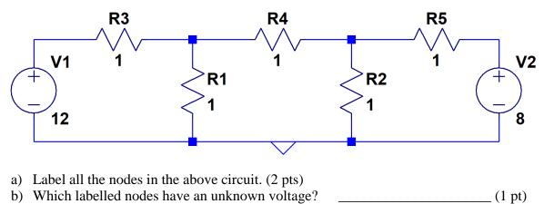
c) Apply KCL and determine the linear system of equations associated with the unknown nodes. (Do not simplify the circuit using parallel and series relationships for resistors.) (3 pts)
