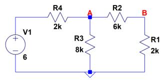
a) Use any method to find the voltages at nodes A and B. (6 pts)
