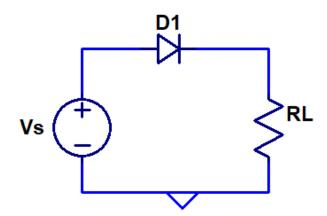
a) For the above circuit, assuming the diode is ideal with VTurn-on = 0V, sketch the voltage across the resistor. (3 pts)
