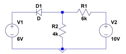
The diode in the above circuit is ideal, with  $V_{Turn-on} = 1V$ . (Same circuit as the previous page.)
