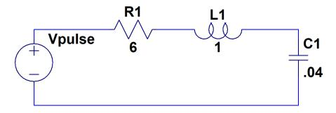
To the best of your artistic ability, sketch the voltage across the capacitor in the above circuit for a pulsed voltage source, between Vmin = 0V and Vmax = 5V. You only need to sketch one 'section' of the decaying sinusoid during capacitor discharge (when the capacitor voltage is decaying to zero). Annotate your plot, indicating 'features of interest'.
