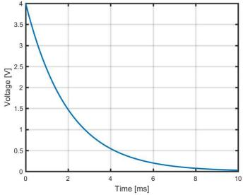
a) For the above plot, determine the time constant in ms. Note, the time axis is in units **milliseconds** (0.001s). (4 pts)
