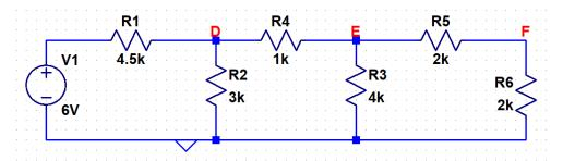
b) Using parallel, series and/or voltage divider concepts, determine the voltage at nodes D, E, and F. Don't make any assumptions based on previous circuits without verifying those assumptions. You can include schematics of circuit reduction techniques for partial credit. (8 pts)
