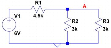
a) Using parallel, series and/or voltage divider concepts, determine the voltage at node A. (4 pts)
