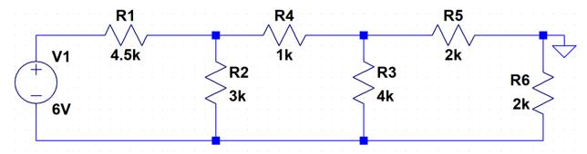
b) The above circuit is the same circuit seen at the end of problem 1, except the ground node has been moved. Determine the voltage across resistor R6. (2 pts)
