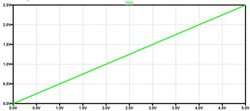
Similarly, the voltage at V1 was set to zero and the voltage V2 was swept from 0 to 5V. The voltage at some node A inside the circuit was measured and the plot of  $V_A$  vs. V2 (with V1 = 0) is shown below.
