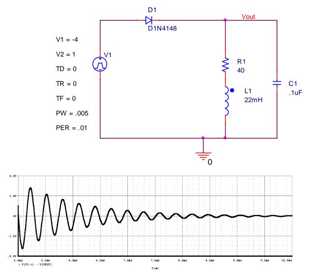
The output voltage clearly shows the behavior we expect from a resonant circuit. Determine the resonant frequency from the plot and from the values of the circuit components. (4pts)
