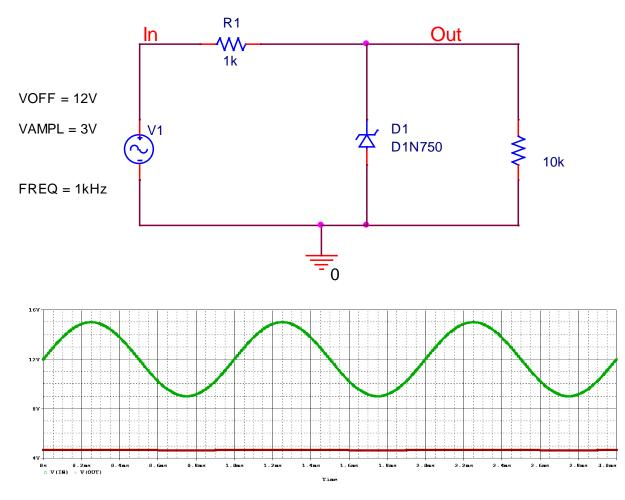
The voltage is about 4.6 to 4.7V. Minimum current  $\approx$  (9-4.7)mA = 4.3mA. PSpice  $\approx$  4mA.
