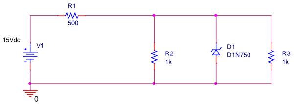
The current through R1 is (15-4.7)/500 = 20.6mAThe current through R2 and R3 each equal 4.7mA The current through D1 is (20.6-9.4)=10.2mAIV=4.7(10.2)=48mW
