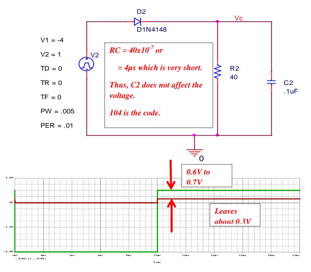
b. The resistance in the circuit above was chosen to represent the resistance of a standard inductor (R1 in the circuit below), which we will now consider. In the data figure, the input voltage and the output voltage Vout are shown for the first half of the square wave
