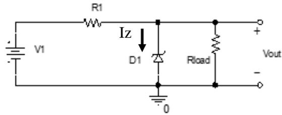
D1 is a Zener. Two different Zener diodes are tried with this circuit. Determine  $V_{out}$ ,  $I_z$  (the current in the Zener),  $I_{R1}$  (the current in  $R1$ ) and the power loss in the Zener for each case. Use the “Some Additional Background” information provided in the crib sheets. (6pts)
