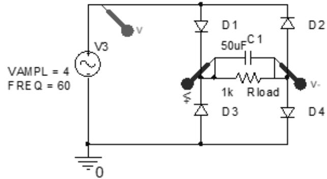
ii. At the time of the peak output voltage, **what is the current in Rload**, (the load resistance)?
