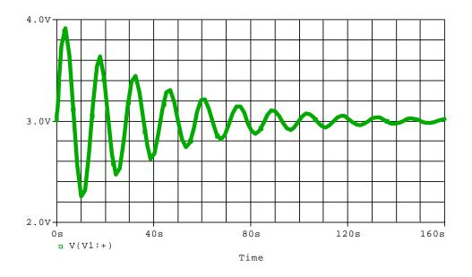
There is a 3V offset given the center of the sinusoid at 3V.
