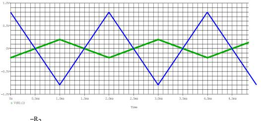
$$V_{out} = \frac{-R_2}{R_1} \cdot 0.2V$$
