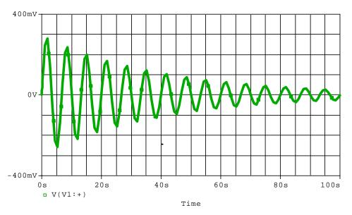
2.1: Find the decay constant,  $\alpha$ , and the angular frequency,  $\omega$ , for this function. Pay close attention to axes. You must label the graph (arrows) with the points you are using for time and voltage for full credit. (6 pts)
