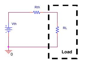
The Thevenin Equivalent circuit consists of a voltage source (Vth) in series with a resistor (Rth), which is then in series with a defined load (RL). Note: A load can be more than one component. If there are mulitple, the value of the load resistance should be calculated to create one component.
