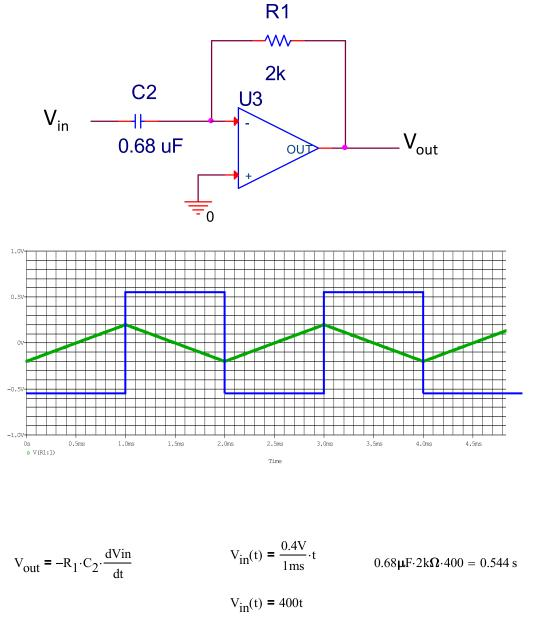
From 0 to 1 +400 slope \* -RC = -0.544 line From 1 to 2 -400 slope \* -RC = +0.544 line
