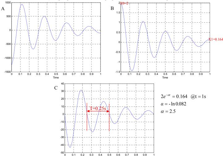
1) (3pt) Identify which plot is **position**, which is **velocity** and which is **acceleration**. From the plots, what are the initial position, velocity and acceleration? Assume SI units (position in meters, velocity in meters per second, acceleration in meters per second squared).
