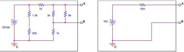
1) (5pt) Find the Thevenin equivalent voltage with respect to A and B for the circuit shown above left.
