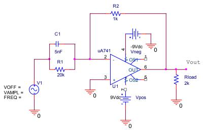
Assume that the input is sinusoidal and we want to find  $H(j\omega)$ , the transfer function, for this circuit. We know that when the non-inverting terminal of an op amp circuit is grounded,  $H(j\omega) = -Zf/Zin$ .
