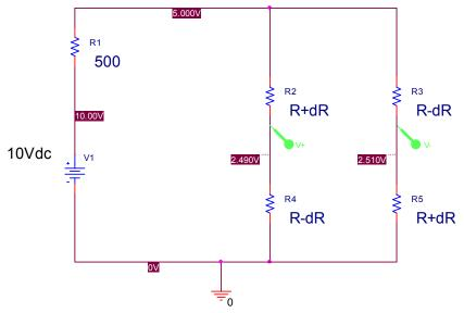
Total resistance in each side of bridge = R + dR + R - dR = 2RTotal resistance of combined sides: 2R||2R = RTo get the top of the bridge to be 5V, with a voltage divider:
