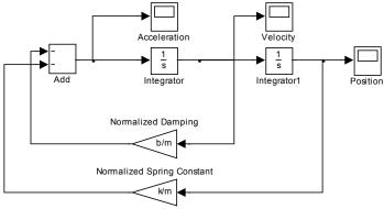
The blocks marked Acceleration, Velocity and Position are 'scopes that provide data on the given parameter as a function of time. In no particular order, these three plots follow for a particular set of values for k, b, and m (the spring constant, the damping constant and the mass, respectively).
