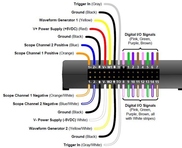
Draw lines between the 2 figures to indicate wires. Both the M2K and the AD2 have the same wiring and colors. W1 is called Signal Generator on the M2K and Waveform Generator on the AD2.
