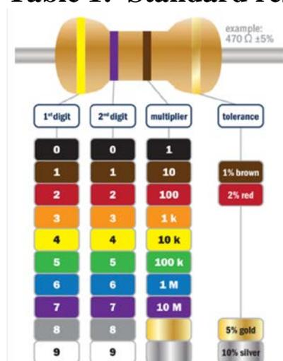
**Figure 1: Resistor color and Tolerance bands**
