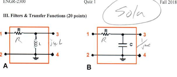
a) Shown above are basic, two-element, passive filter configurations made with RL and RC combinations. Determine the general complex transfer function for each circuit in terms of R, L, C and frequency  $\omega$ , by modeling each as a voltage divider. This is an AC steady state problem. (2 pts)
