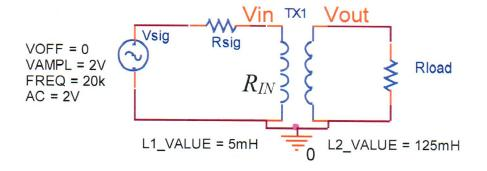
Given the circuit above with Rsig=100 $\Omega$ , and Rload=5k $\Omega$ , assume an ideal transformer with full coupling.
