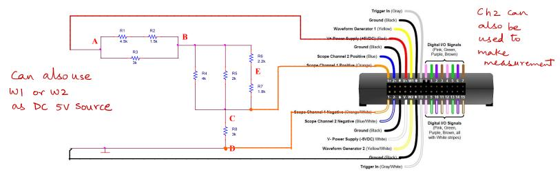
f) What voltage will be measured in part e, i.e. across R<sub>8</sub> using the Analog Discovery? Give your answer in Volts. Hint: Add the input resistance of Analog Discovery channel. (3
