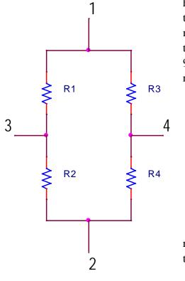
have such a bridge but we do not know the value R of the resistors, so the following resistance measurements are made across each pair of adjacent terminals:  $R_{14} = 90\Omega$ ,  $R_{42} = 90\Omega$ ,  $R_{23} = 90\Omega$ ,  $R_{31} =$  $90\Omega$ . Use the measured values to determine the resistance of R. (4 pts)
