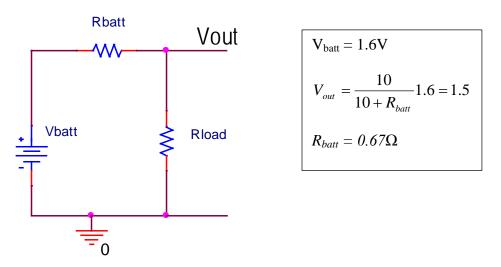
d) Find the power delivered to  $R_{load} = 10\Omega$ . Will a <sup>1</sup>/<sub>4</sub> Watt resistor be adequate for this measurement or will a <sup>1</sup>/<sub>2</sub> Watt or 1 Watt resistor be required? (4 pts)
