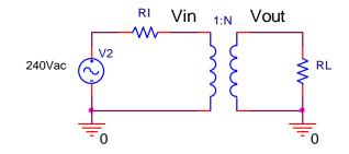
1) Given the circuit above, assume an ideal transformer with full coupling. With  $RI = RL = 100\Omega$  and N=1, find Vin, Vout, and the power in RL. (6 pts)
