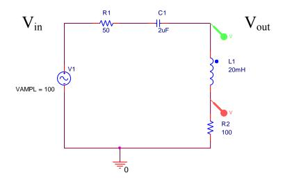
For this circuit,  $V_{in}$  is the voltage source and  $V_{out}$  is the voltage across the series combination of the inductor and resistor.
