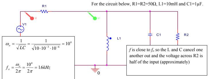
1) Which of the 3 graphs below would best represent the output seen across resistor R2; where  $Vin = 10V \cos(2\pi ft)$ , with f = 1kHz? (8 pts)
