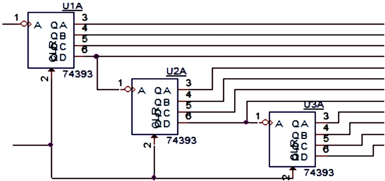
c. (3 pts) Above, a circuit is shown consisting of several counters combined. What is the largest number that can be represented using this counter circuit?
