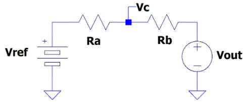
$V_{ref}$  is a dc voltage so it is shown as a battery.  $V_{out}$  has various values so it is shown as a voltage source.
