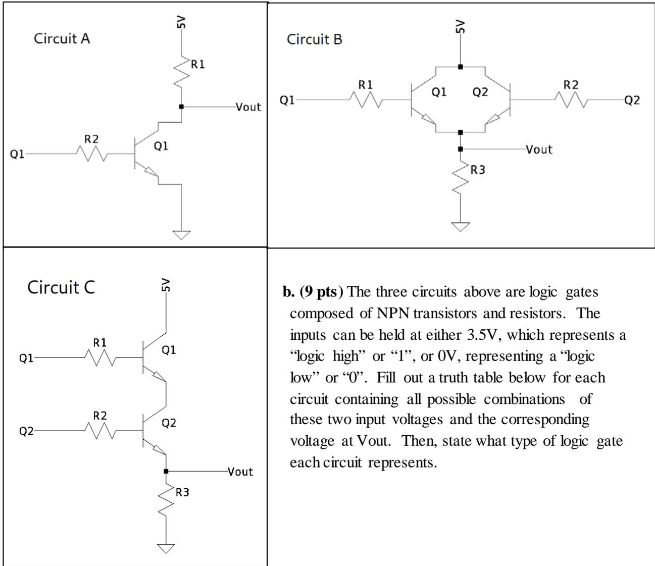
**b. (9 pts)** The three circuits above are logic gates composed of NPN transistors and resistors. The inputs can be held at either 3.5V, which represents a “logic high” or “1”, or 0V, representing a “logic low” or “0”. Fill out a truth table below for each circuit containing all possible combinations of these two input voltages and the corresponding voltage at Vout. Then, state what type of logic gate each circuit represents.
