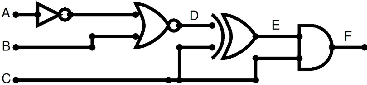
a. (4 pts) Fill out the truth table below. Start by writing all possible combinations of the inputs A, B, and C. Then determine the corresponding outputs D, E, and F.
