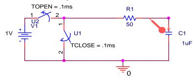
That is, a 1 Volt DC source has been connected across a resistor-capacitor combination as shown. At time t=0.1ms, the source is disconnected from the circuit and the resistorcapacitor combination is shorted to ground. When this occurs, the voltage across the capacitor decays to zero. Assume that you have measured the following:
