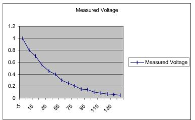
where the time scale is in microseconds. Note that the voltage drops from around 1Volt to a little less than 0.3Volt in about 50 microseconds. Thus, for exponential decay, the time
