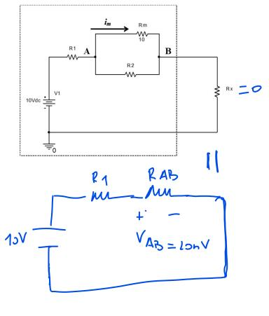
Using voltage divider and your previous findings, develop a relationship between R1 and R2 for case 1
