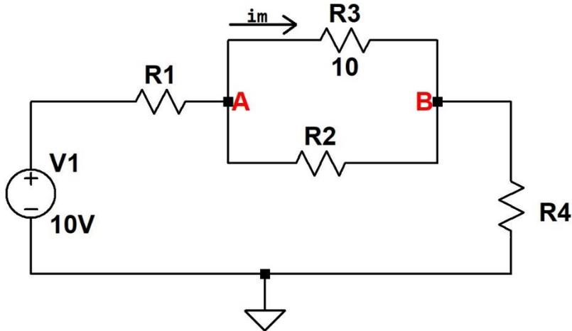
**Case 1:** Given that when  $R_4 = 0$  ohms, the current through resistor  $R_3$  is 2 mA, i.e.  $i_m = 2$  mA.
