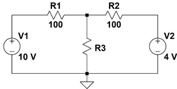
**Part a)** (10 points) Determine the value of resistance  $R_3$  using nodal analysis such that the voltage across it is 6 V. Show handwritten work.
