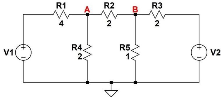
Using nodal analysis techniques, express the voltage at node A and node B in the form,  $V_A = aV_1 + bV_2$  and  $V_B = cV_1 + dV_2$ . In other words, find values for the constants a, b, c, and d.
