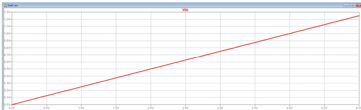
Figure B-3. Voltage at B as a Function of Source Voltage V1 (V2 = 0)
