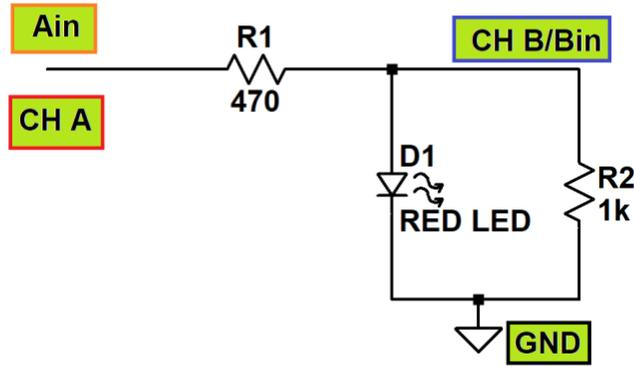
1. Using the process described in the video titled “Source and Measure DC Voltages”, configure Channel A (**CH A**) as a variable DC voltage source and the **Ain** pin as the DC voltmeter. The value of the DC voltage source will be adjusted to make multiple measurements. **Note, here CH A needs to be in Split I/O mode. Watch video for the details.**
