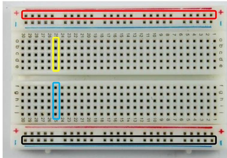
If you purchased the Analog Devices parts kit, the included protoboard is shown below. In this case, the power buses are not part of the board. Only the banks of five holes on either side of the chip gap are available as shared connected holes.
