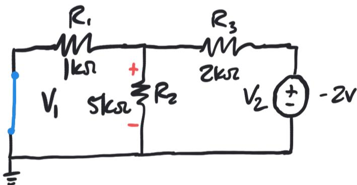
$$V_{R2,V2} = (-2V) \cdot \frac{R_1 \parallel R_2}{R_3 + R_1 \parallel R_2} = (-2V) \cdot \frac{0.833k\Omega}{2k\Omega + 0.833k\Omega} = -0.588V$$
