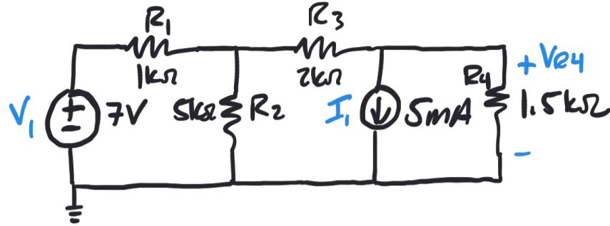
1.  $V_{R4}$  due to  $V_1$ :
