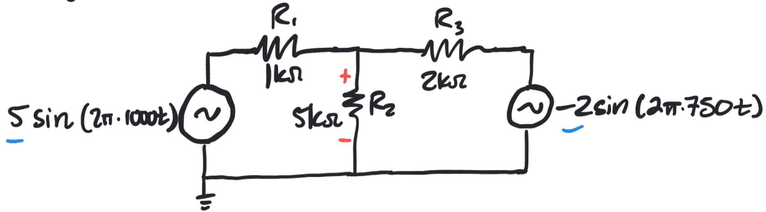
• Solve for  $V_{R2}$  using Superposition
