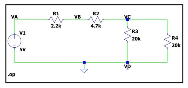
Here we have a simple circuit with resistors **R1** (2.2 k $\Omega$ ) and **R2** (4.7 k $\Omega$ ) in series with a loop containing resistors **R3** and **R4** (20 k $\Omega$  each) in parallel. The circuit is powered by a 5 V DC voltage source **V1**, and nodes **VA–VD** are labeled to show where our voltage readings are taken.
