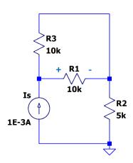
$I_{R1}=rac{I_S}{2}$  due to the current divider between R3 and R1 (since R1 and R3 are equal, equal amounts of current will flow through each.
