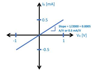
**1.2** [2 pts] The transfer characteristic for an amplifier circuit is shown to the right. What type of amplifier is this? What is its gain?
