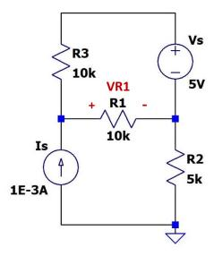
a. [3 pts] Find  $V_{R1}(V_s)$ , the voltage across R1 due to  $V_s$  only.
