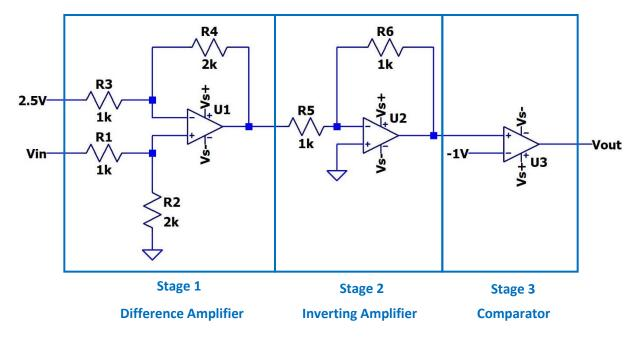
a. [3 pts] Identify how many stages are in this op-amp circuit. Draw a box around each stage and label them "Stage 1", "Stage 2", etc.
