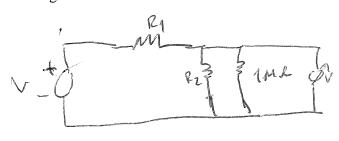
**Part b)** (10 points) Draw an equivalent circuit that includes the resistance of the voltmeter. Compute the effective resistance of R2 and the resistance of the voltmeter for R2= 100  $\Omega$ .
