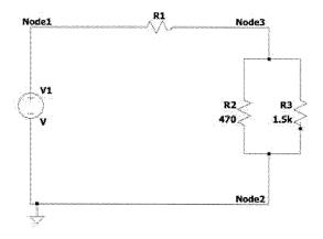
a. (7 points) The voltage drop across R1, R2, and R3 is to be measured using the M1K board by making wire connections between the circuit and M1K board pinouts. You would also need to use the M1K board to supply 4V for the voltage source V1.
